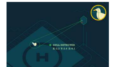
The system determines the exact location of the bird and fires a targeted laser project
